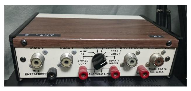
Three SO-239 connectors are available for three antennas using coaxial cable. Connectors labeled COAX 2 and COAX 1 can be connected directly to the transmitter via the switch shown above or switched to use the tuner circuitry. The BYPASS COAX connector cannot be routed through the tuner circuitry. You can use this for a dummy load or I use it for my tri-band beam that doesn't need the tuner. There are also outputs for a balanced line or a single wire antenna.
